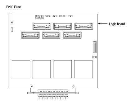
Figure 4-1: Fuse location on the TMSPGC probe adapter
