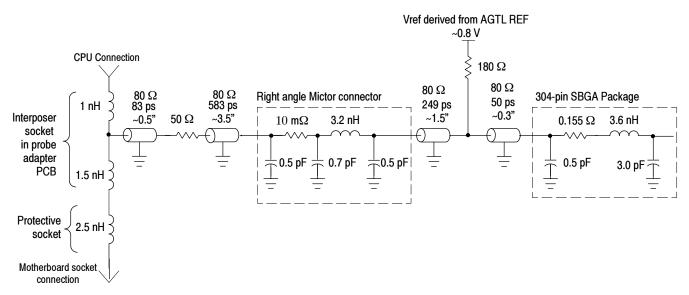
Figure 3-2: AGTL signals with active loads, except RESET#
