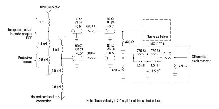
Figure 3-1: BCLK and BCLK# signals with active loads
