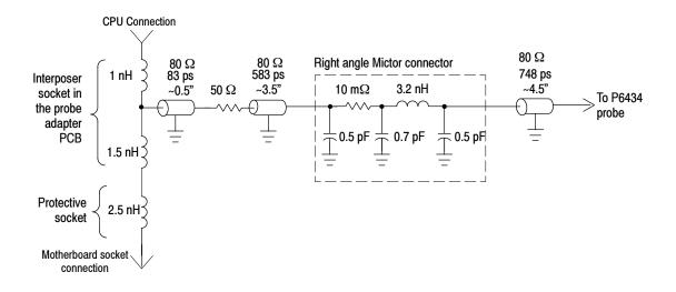
Figure 3-4: JTAG signals without active loads
