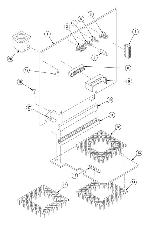
Figure 5-1: Exploded view of the TMSPGC PGA370 probe adapter
