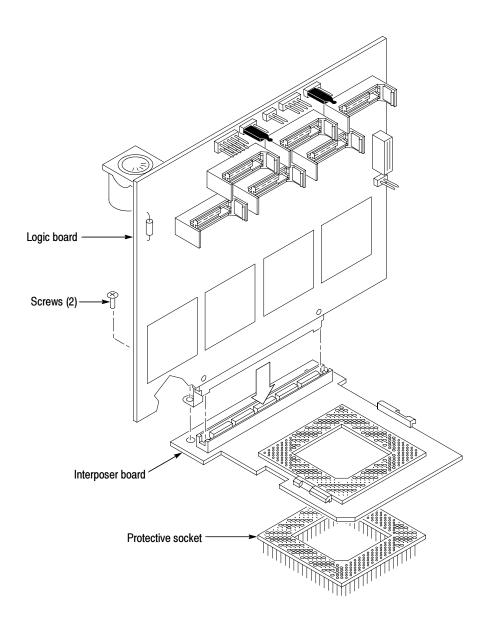
Figure 1-2: Attaching the Logic board to the Interposer board
