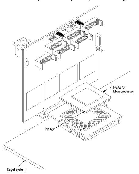
8. Insert the microprocessor into the probe adapter as shown in Figure 1-6.
