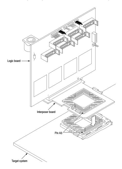
Figure 1-5: Inserting the probe adapter into the socket
