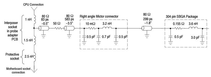
Figure 3-3: CMOS signals with active loads, plus RESET#
