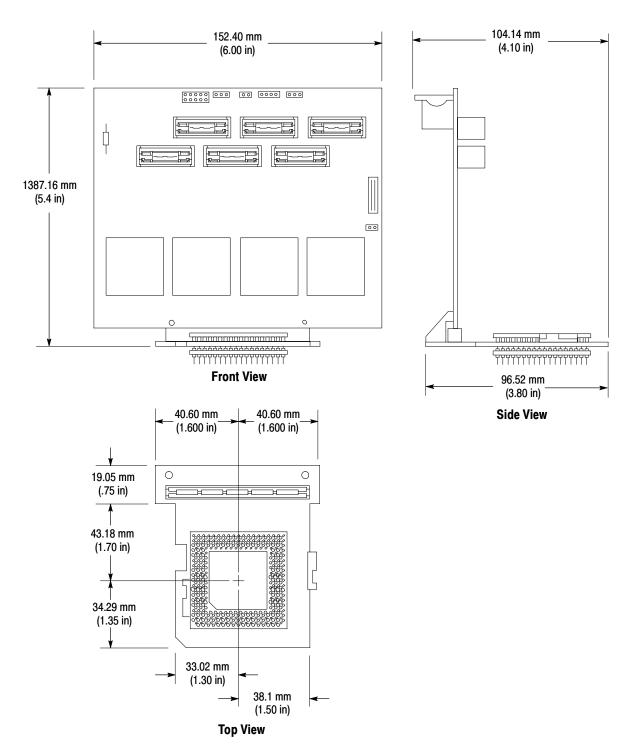
**Dimensions** Figure 3-6 shows the dimensions of the TMSPGC probe adapter.
