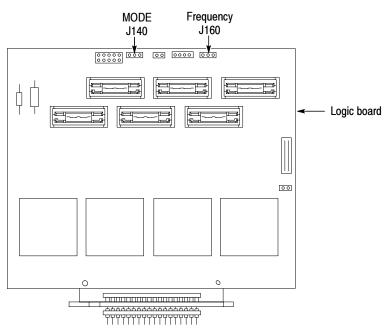
Figure 1-8: Jumper locations on the TMSPGC probe adapter
