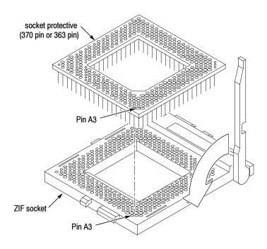
Figure 1-4: Inserting a protective socket into the ZIF socket
