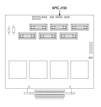
Figure 1-10 show the APIC bus signal pins for the TMSPGC probe adapter.
